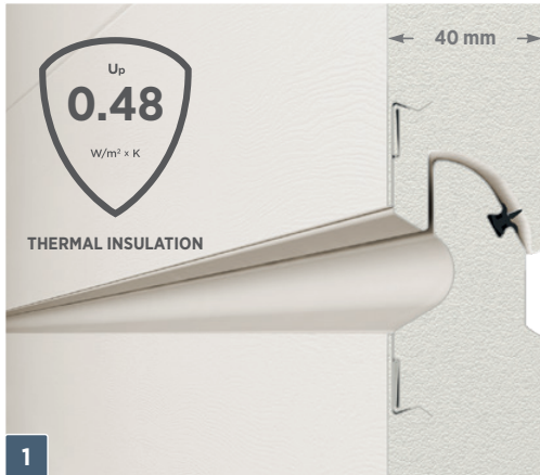
1 Door leaf – made of 40 mm thick sectional panels and filled with freon-free polyurethane foam. Thermal transmittance factor of the panel U_p = 0.48 [W/m 2 xK].
