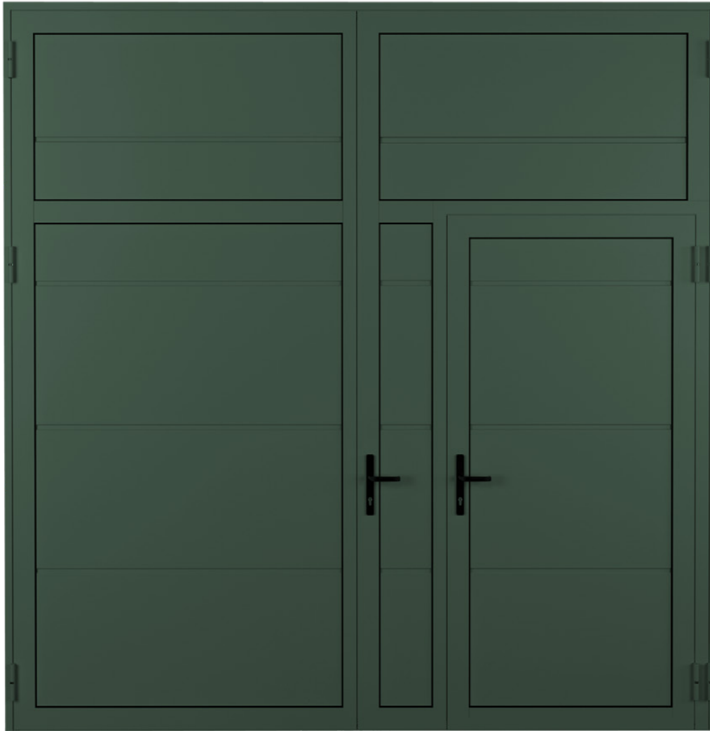
PRESTO 50 double-leaf door with a wicket door - the door with a height of H_o \geq 3,000 mm or fitted with a wicket door also features a horizontal reinforcing crossbar at the height of 2,087 mm
